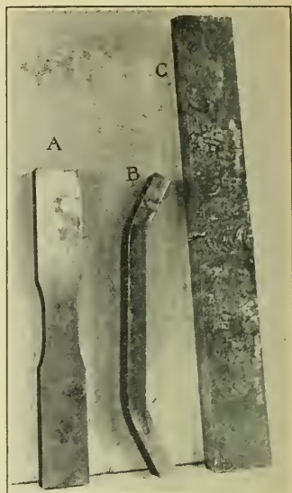
FIGURE 2 — The Company's standard test coupons: (A) Tensile Test; (B) Free Bend Test for Ductility; (C) Nick Break Test for Soundness.
